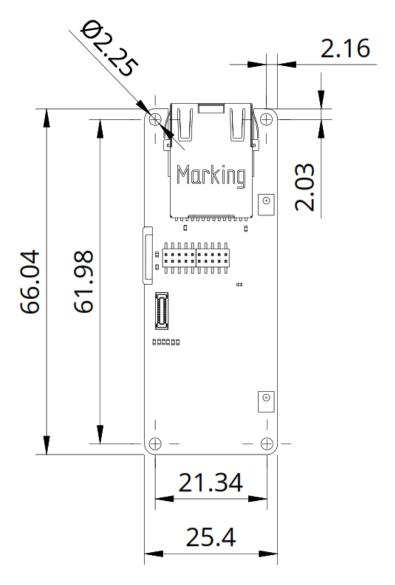
The Portenta Vision Shield has four 2.25 mm drilled mounting holes for mechanical fixing.
